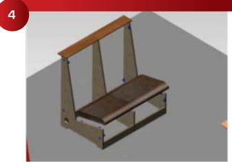
Firmly push the panels into place to mark the 334 Mounting Screw locations. Install the mounting screws using a 913 Brad Point Drill Bit, 5mm.
