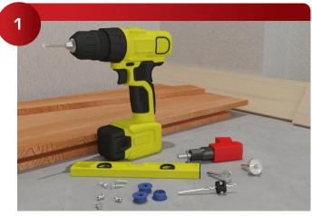
320 Zero, 330 Alignment Pins, 349 Upholstery Mount, 910 Forster Drill Bit 1",913 Pilot Drill 5MM & Stop, Dead Blow Hammer or 305-320 Hammer Head for Zero, Panel Adjuster, 1/32" plastic laminate, Spray Contact Cement, Panel Adhesive
