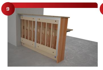
The 320 Zeros have a 1/40" rim, the thin reveal laminate can be 3 ply plywood or horizontal grade plastic laminate. Reveals can be quickly fit and installed.
