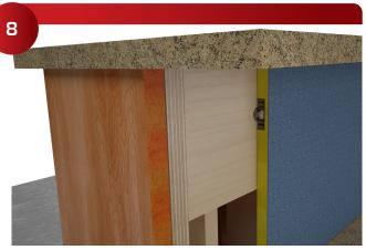
The back panel is a 1/2 thick high-density mineral board core tackable fabric wall panel. The soft cores generally requires the insert be installed with epoxy poured around the core to make the panel removable.
