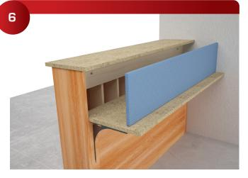
Carefully push the panel into the 330 Zero Alignment Pins to mark the Zero's mounting screw locations. If needed install the reveal laminate in the reveal locations as needed.
