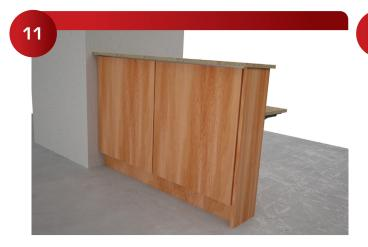
Push the wood panels straight into place, panels can be eastly removed with a glass suction cup, or a plastic pry bar.
