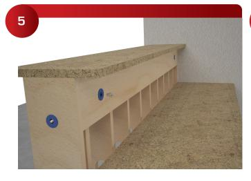
Place 330 Zero Alignment Pins on each individual panel's set of inserts (the Alignment Pins are reusable).
