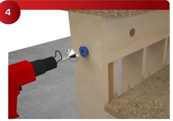
You can use a dead blow hammer or pneumatic hammer to insert the 320 Zero at all corners of the panels to install the inserts.
