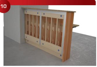
Carefully push the panels into the 330 Zero Alignment Pins to mark the Zero's mounting screw locations. Next drill the 5mm holes for the 334 Mounting Screws in the position indicated by the alignment pins.
