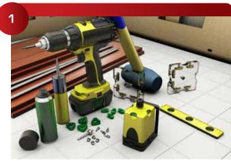
Required Tools; 300 Green Glide, 318 Drill Template, 311 Alignment Pins, 913 Pilot Drill, 5MM Center Point Drill & Stop, Dead Blow Hammer or 305-300 Hammer Head for Green Glide, Panel Adjuster, 1/32" plastic laminate, Spray Contact Cement, Panel Adhesive.
