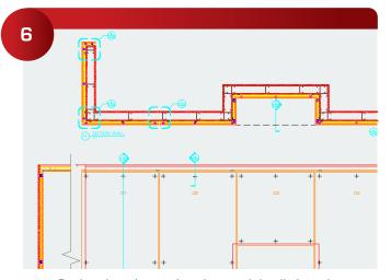
Revise shop drawn elevations and details based on the field verified horizontal and vertical level lines, end conditions, field changes, etc..
