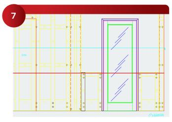
Revise shop drawings to reflect face of all panel sizes on primary drawing layer. Revise the furring layer to match panel sizes precisely, this a critical step.
