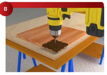
It is helpful to set the 334 Mounting Screw 1-3/4" to 2" from panel corners to simplify mounting screw locating. (**Useful Accessories:** The 318 Drill Template, 2" Offset (includes Template & Stops) helps speed this process.)
