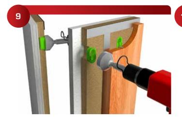
Install the 300 Green Glide using a Dead-Blow Hammer. (**Useful Accessories**: The 305-300 Hammer Head can speed up installation of the 300 Green Glide inserts.)
