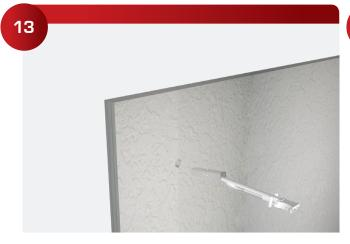
Install the 250 Snaptoggle into the sheetrock, pull back the straps and firmly push the plastic ring into the hole. Break off the plastic straps flush with the wall surface.
