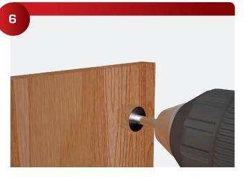
320 Zero should be drilled about 2" off the panel corners to firmly hold the panels. Drill the holes with a 1" Forster bit, 7/16" deep (in the field) or with a CNC (in the plant).
