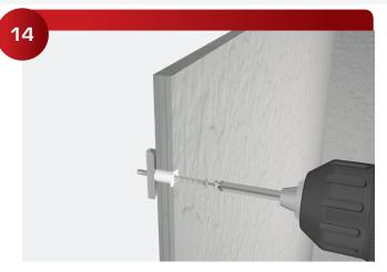
Add the provided 1/8" Nylon washer to 245 Mounting Bolt and screw into 250 Snaptoggle. (**TIP:** Do not over tighten the bolt, it can compress into the Sheetrock.)
