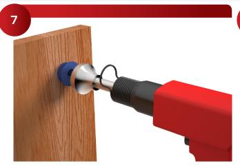
Install the 320 Zero using a Dead-Blow Hammer on a solid work surface. The 320 Zero protrudes 1/32" allowing the panels to be packed flat for shipping. (**Useful Accessories:** Star Hanger has the 305-320 Hammer Head for quicker install of the 320 Zero.)
