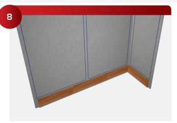
Install the baseboard or a level reference board to steady the panels on while marking for the 245 Mounting Bolt. The reveals can be quickly painted, or you can use 1/32" plastic laminate with contact cement.
