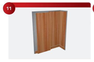
Set the panels on top of the reveal strips and push them firmly into the drywall to mark the locations for the 245 Mounting Bolt.
