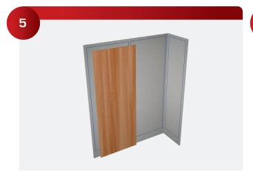
Field verify the face of panels sizes based on horizontal & vertical layout lines. Write the panel numbers on the walls.
