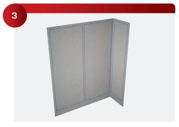
Layout the perimeter of the panels on the walls with a blue chalk line. Confirm that the panel layout is workable with field alignment, electrical and any other requirements.
