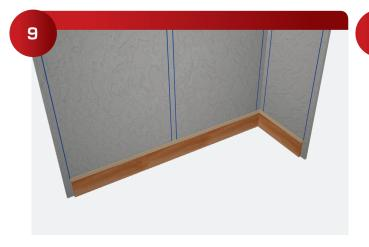
Cut several reveal strips the same width as the reveals between the panels. Use these as shims to temporary hold the panels in place for marking.
