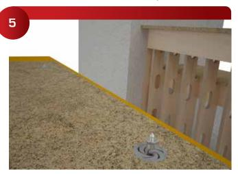
If prepared in the field, place 229 Galaxy Alignment Pins in each 225 Galaxy to mark in the furring. The Alignment Pins are reusable.
