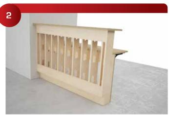
Determine the location of the panels and install a 225 Galaxy in the die wall as needed. All the die wall parts and panels can be pre-machined on a CNC.
