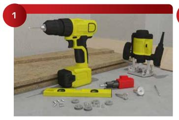
Required Tools; 225 Galaxy, 234 Euro Screw, 229 Galaxy Alignment Pins, 916 Drill Collar and 516 Center Drill, 911 Carbide Tipped Drill 1-1/4", Galaxy 1-1/4" Template, 915 Router Bit, 3/32" Offset
