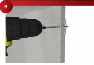
Install 952 Pop Toggle and 236 Combination Screws. Push red the setting stick into the 952 Pop Toggle to force the arms to pop out in the back. Using a drill set on low torque gently snug the screws. (TIP: Do not over tighten the screw, it can compress into the sheetrock.)
