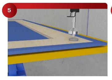
Install the 224 Galaxy flush with the panel surface using a Dead-Blow Hammer.
