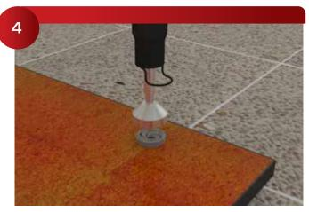
The 226 Galaxy can be plant installed flush with the back of the sign, allowing signs to be shipped flat with the hardware installed. A plant prepared CNC cut sign and layout template, including the centers for the mounting screws, makes the field installation very quick.
