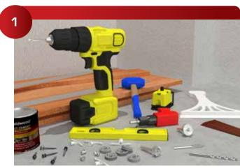
Required Tools; 225 Galaxy, 229 Galaxy Alignment Pins, 236 Combination Screws, Dead Blow Hammer or 965 Galaxy Hammer, 919 Carbide Tipped Drill 5/16", 911 Carbide Tipped Drill 1-1/4", Forstner Drill, 952 Pop Toggle.
