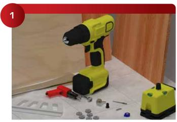
Required Tools; 226 Galaxy, 229 Galaxy Alignment Pins, 239 Machine Screws, Dead Blow Hammer or 965 Galaxy Hammer, 917 Drill & Tap combination, 10-24 Thread, 911 Carbide Tipped Drill 1-1/4" Forstner Drill
