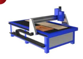
The panels and template can be cut out with a CNC router. Or the same template can be used with the 916 Drill Collar and 5/16" Center Drill to mark the location of the 1-1/4" Forstner Drill.
