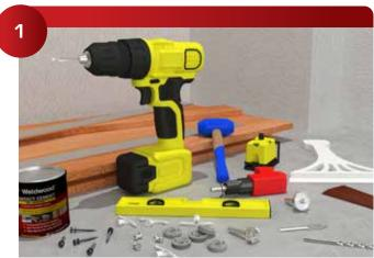
Required Tools; 225 Galaxy, 229 Galaxy Alignment Pins, 236 Combination Screw, Dead Blow Hammer or 965 Galaxy Hammer, 919 Carbide Tipped Drill 5/16", 911 Carbide Tipped Drill 1-1/4" Forstner Drill, 952 Pop Toggle, 920 Panel Adjuster, 922 Vacuum Cup 8", 1/32" plastic laminate, Contact Cement.
