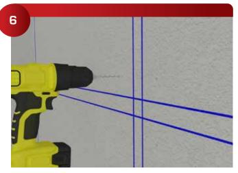
Screw the template in place and drill the 919 Carbide Tipped Drill 5/16" Bit slowly through the sheetrock. (Tip, the hole needs to be clean to hold the Pop Toggle accurately).
