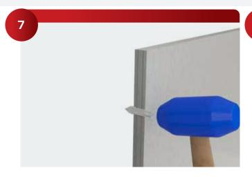
Install the 952 Pop Toggle into the sheetrock, it should fit firmly.
