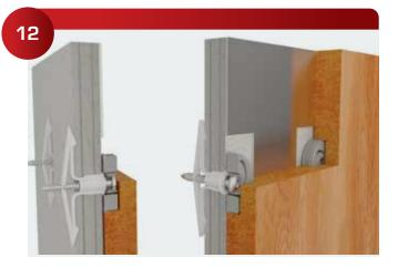
Cutaway view of the assembly
