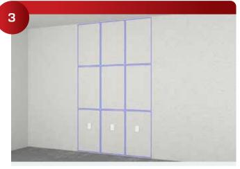
A full layout is not required; you just need the layout required to install the reveal strips. Adding a support strip under the template is helpful.
