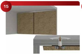
There should be about a 1/8" gap between the sheetrock and the Solid Surface panel. The 225 Galaxy only holds the panel in place until the silicone sets.
