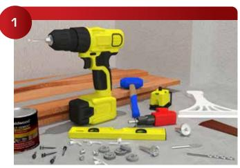
Required Tools: 225 Galaxy, 236 Combination Screws, 229 Galaxy Alignment Pins, Dead Blow Hammer or 965 Galaxy Hammer, 919 Carbide Tipped Drill 5/16", 952 Pop Toggle, 920 Panel Adjuster, 922 Vacuum Cup 8"
