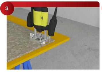
The 225 Galaxy can be CNC cut and plant installed flush into the pre-engineered solid surface panels, allowing the panels to be shipped flat packed.
