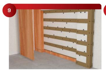
Place reveal spacers between panels to locate the exact panel positions. Carefully push the panel into the 211 Alignment Pins to mark the Lock positions.
