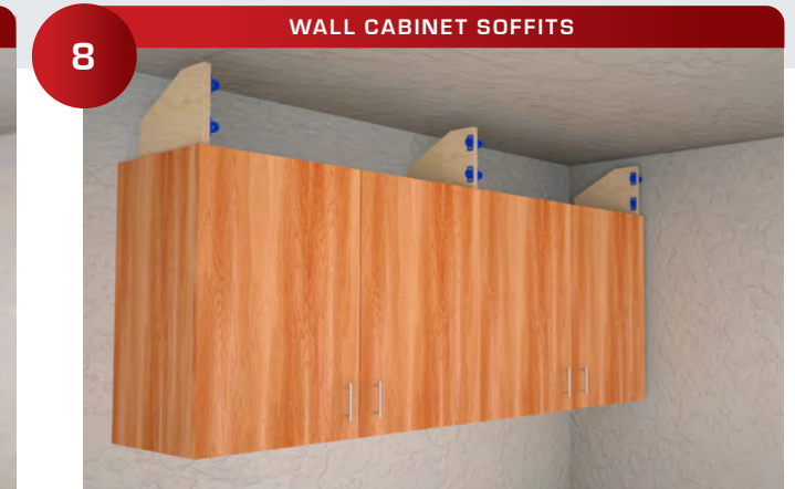
Install wall gussets above the wall cabinets with the 325 Zero Side Mounts pre-installed. The gussets can be installed by simply sitting them in beads of panel adhesive and allowed to dry overnight.
