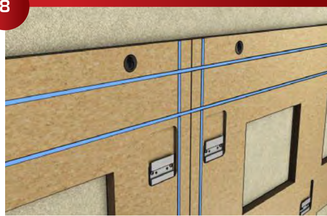
The position of the reveals can be marked with the CNC in the shop.
