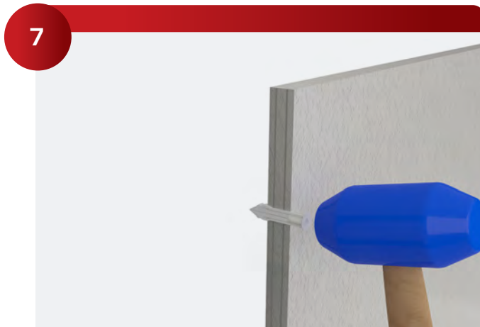
Install the 952 Pop Toggle into the sheetrock, it should fit firmly.
