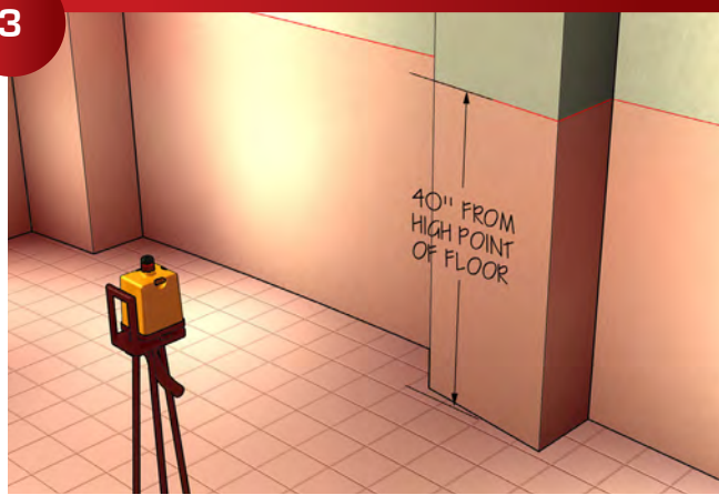
Find high point of floor, check to see if the project has a pre-set horizontal bench mark. If not set your own horizontal bench mark.
