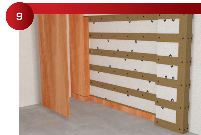
Place reveal spacers between panels to locate the exact panel positions. Carefully push the panel into the 211 Alignment Pins to mark the Lock positions.
