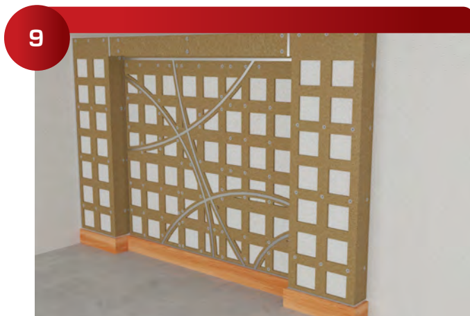
Install the baseboard
