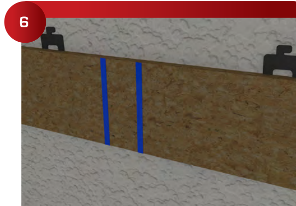
6 Transfer the revised shop drawing panel sizes to the face of the furring.
