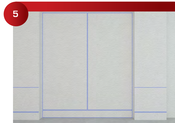
5 If the project is simple, shimming out the 430 S Clip Bars works well. If the panels have other constraints, you need to be careful. There are many possible conflicts when shimming bars out large areas, panel alignments, widths of door jambs, electrical build outs, held dimension are just a few examples.
