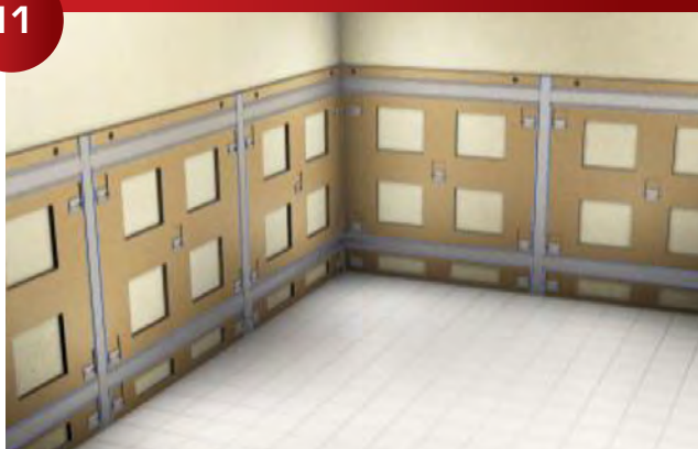
When using pre-engineered furring your panel clips should fit 2" down from the top and corners.
