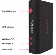
This package does not include the 18650 cell or charger. Customer need to choose suitable 18650 cell and the corresponding charger. The cell output should be 30A or above.
