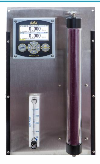
ammonia and sodium are removed while mineral salts such as chloride and sulfate are converted into more conductive acids. Utilizing a well-proven algorithm, a pH measurement can also be determined from specific and cation conductivity values for systems utilizing ammoniated chemistry.
