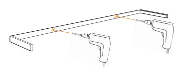
USE 1/4" LAG BOLTS, 3" LONG, TO SECURE THE INNER METAL BRACKET TO THE WALL. THERE SHOULD BE NO MOVEMENT WHATSOEVER ONCE THE BRACKET IS SECURED.
