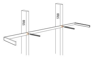
USING A 3/8" DRILL BIT, DRILL A HOLE THROUGH THE METAL BRACKET WHERE THE STUD WILL BE LOCATED. THE METAL BRACKET REQUIRES A DRILL BIT SPECIFICALLY DESIGNED FOR METAL MATERIALS.
