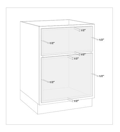
Measure the height and width of the opening of the cabinet frame that you want the front to cover. Add 1" to the height and 1" to the width to account for the overlay.
