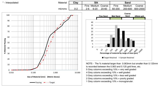
This information is a guide only and does not constitute a specification. There are a vast number of sands differing in grading and qualities. To be sure that a well graded sand is being used it is necessary that at least four grades form a substantial part of over 10% of the proposed sand. This sand has 4 grey columns in the size range above 10% indiciating a well graded sand.
