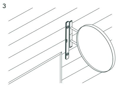
Firstly, you need to mark out the screw positions. Using a level, place the sign in its desired position, and while someone holds it straight, use a pencil to mark where the 6 x screw holes will go. Drill the holes with a drill bit to suit.
