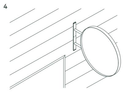
Using a screwdriver, fix the screws into the 6 x screw holes using the concrete or wood screws supplied.
