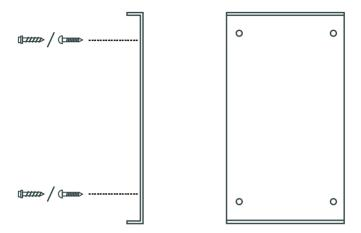
Select a space to install your sign. The sign should be fixed into studs or a solid wall. Depending on the wall, pick between the wood screws or the concrete screws. Make sure the bracket is in portrait orientation. Use a level to get the bracket straight and fasten the screws with a drill. Put a screw in each of the four holes.
