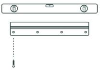
Once selected the wall space, fix the first screw into the bracket on one end then, using a level to ensure it will sit straight, ensure the other 3 screws all go in perfectly horizontal to one another.
