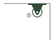
Install Pulley 3 further back from pulley 2, close to the Corner of the ceiling and wall. Ensure all three pulleys are perfectly aligned.
