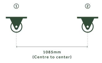
Install pulley **2** 1085mm back from pulley **1**. Ensure they are perfectly aligned.
