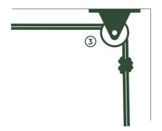
Raise the Hanging Drying Rack to the desired height attended for use (chest height recommended). Tie a knot in the two ropes just behind pulley (3). This stops the rack from lowering any further. Tie off rope around the cleat. Cut any excess rope off and melt the ends for a clean and tidy finish.
