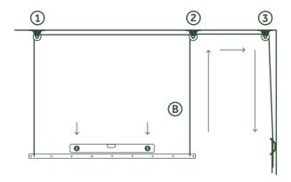
Thread Rope (B) through Pulley (2). Continue across and through pulley (3). Pull both ends of rope (A+B) until the Hanging Drying Rack is raised off the ground. Adjust each end accordingly until the rack becomes level in the air - A builders level should be used for complete accuracy.
