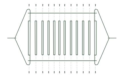
Once you are happy your Hanging Drying Rack is in the correct position place the dowels in the middle evenly so they match up to the correct holes on the outside brackets, using the Allen key to tighten the smaller screws.
