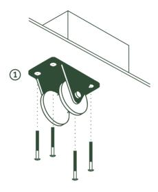
Screw Pulley 1 into the ceiling. Make sure the pulley is secured to a beam.
