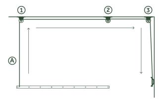
Thread Rope A through Pulley 1. Continue across to pulley 2 and then through pulley 3.
