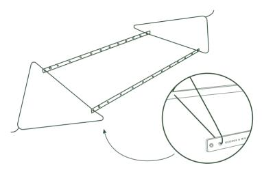
Please ensure that the logo is facing outwards when positioning the frame for assembly.
