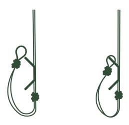
To keep excess rope out of reach, loop the rope up over the cleat.
