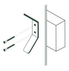
Install the Rope Cleat vertically below pulley 3 on the wall. Please ensure the screws find a stud. All three pulleys and the rope cleat must be aligned.
