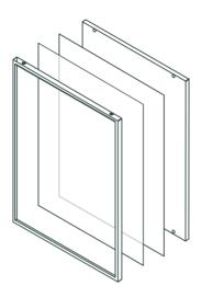
Once you have the mounting bracket fastened to the wall, you can then place the printed paper, clear acrylic, and frame together ready to bolt together.
