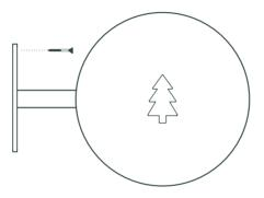
Select a space to install your Medium Round Sign, somewhere unobtrusive and highly visible. We recommend fixing the Medium Round Sign into studs or a solid wall. Insert the first screw using either the concrete or wood screws provided depending on your installation surface.
