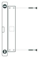
Using a level, position the sign so it is perfectly vertical. Fasten the remaining screws to ensure the Medium Round Sign is securely fixed to the wall.
