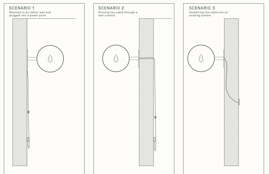
If the Light Box is mounted indoors and the electrical cable is visibly running down the wall to a power point, you have the option to install it yourself.
