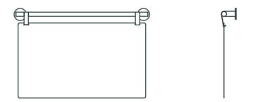
The Ceiling Menu Board isn't just for hanging from the ceiling! You can also mount it on your wall. If you are mounting onto a drywall, it will need to be fixed into a wooden stud to make sure it is properly fixed.
