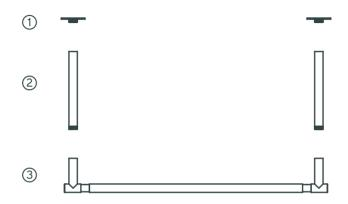
Thread the ceiling mounts (1), rod extensions (2), and hanging frame together (3).
