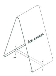
Remove the rubber foot from the nut and bolt and place the bracket to the middle fixing points of the sign using the nut and bolt from the rubber foot.
