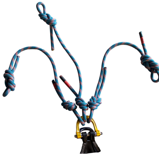
Traditional (2 x Long & 1 x Short Loop) Cow's Tail Arrangement. Re-threaded figure of 8 to Harness Attachment Ring & Re-threaded figure of 8 End Terminations
