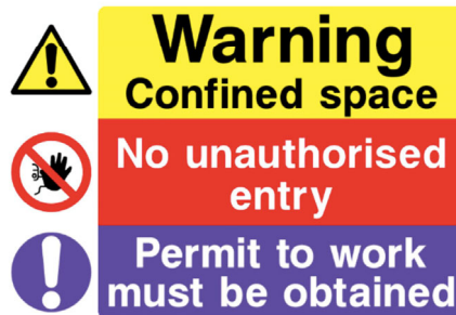
Typical 'Permit to Work' Signage
