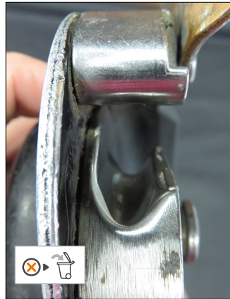
• Cam groove worn to wear indicator
