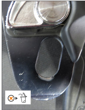
• Attachment hole deformed by a shock load
