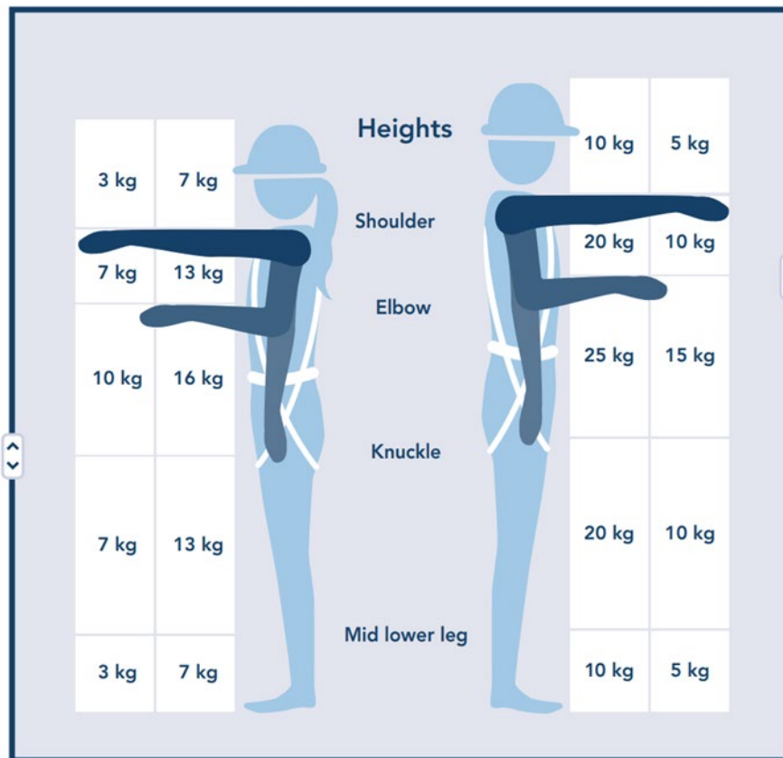
Figure Annex 5.1 - Lifting and lowering filters
