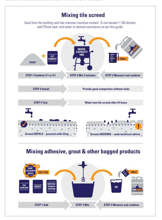
Efflock is a high performance, water based, VOC free, liquid additive designed for the bulk impregnation of cement based building materials to prevent efflorescence and damp.
