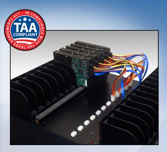
This TAA Compliant Hard Drive Duplicator is easy to use, and can clone up to 23 hard drives or solid state drives simultaneously. As a stand-alone unit without the need to connect to a computer, the KanguruClone 23HD SATA Pro Drive Duplicator is perfect for large duplication jobs.
