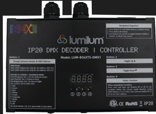
DMX1 Decoder/Controller (IP20 Rated/Indoor) LUM-B34XTS-DMX1
