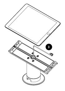
Plug the provided lightning cable into the iPad, and feed the USB end through the center of the stand.
