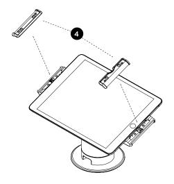
Place the iPad into the Lock Belt and place the End Caps ensuring that all parts fit together with no gaps.
