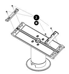
Unscrew the 4 screws using the tools provided, and remove the end caps.  $\,$
