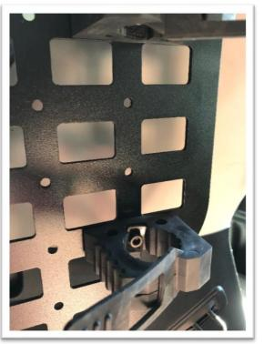
7. Now install the largest spacer and longest bolt at the back of the panel. Closest to the passenger seats.
