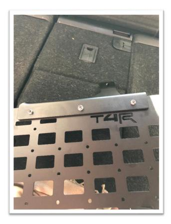
5. Using the factory bolt mount up the storage panel. Start by threading the bolt half way.
