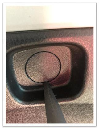
3. Moving on to the coat hanger rack up top. Use your plastic pick and pop open the hanger. Using a ratchet, remove the 10mm bolt set this aside as you will be re using it.
