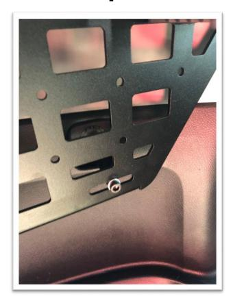
8. Grab the second largest bolt and spacer and install it in the mount closest to the tail light.
