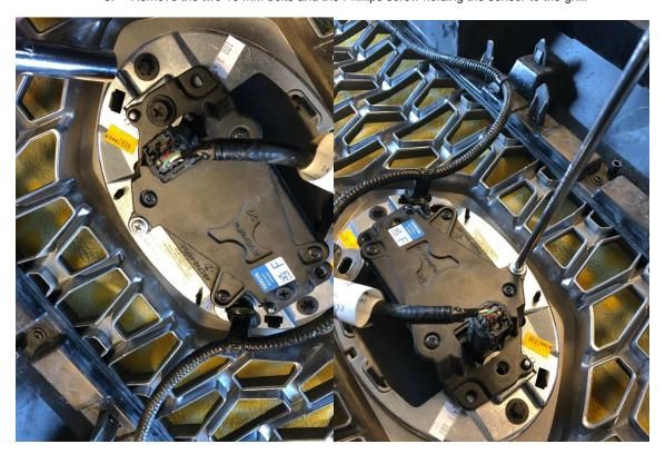
6. Using the Philips head screw driver remove the screws attaching the bezel.
