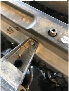
2. Then using your flat headed screw driver pop the push clips up and pull out.
