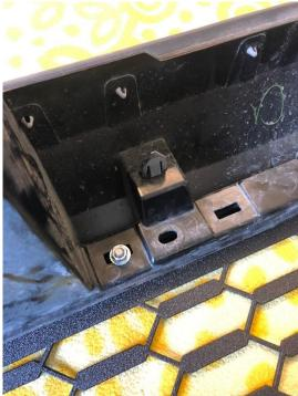
10. Once you have all the nuts on, leave them loose and position the grill as best you can. Flip it back over and snug the bolts up using 10mm ratchet. You are just snugging these up almost just to the point where the washer won't move. If you over tighten it can cause dimpling in the paint. You might find it easier to use a 10mm wrench on the end bolts.
