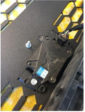
12. Place the washer on like the photo. It should have the thinnest side at the top and the larger side at the bottom. Make sure it is even and straight as best as you can.
