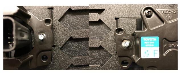
Tight up without moving the spacers or the sensor.
