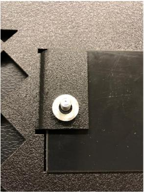
When putting the sensor on, push it all the way to the top of the grill. You don't want the sensor to pick up the bottom edge of the grill.
