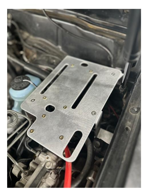
6. When ready install the fuse block and breaker with a 2.5mm Allan key.
