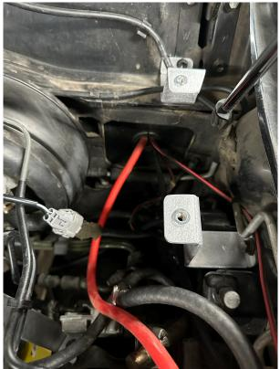
3. Lastly install the longest bracket. You only need to loosen the 12mm bolt and slide the bracket into place. You will need a long extension to reach the bolt. It is directly across from the top shock mount bolt.
