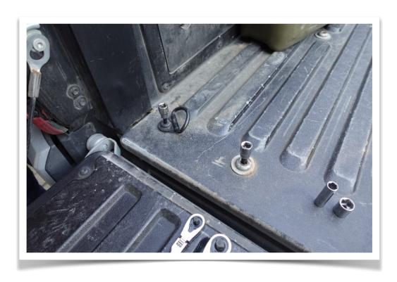
2. Next install the bed stiffer with the two bolts you just removed. Tighten down the bolts and mark/punch the three holes. (Make sure the bed stiffer is tight against the truck).
