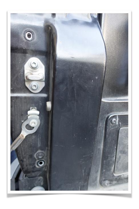
5. You can now drill the holes starting with a smaller pilot bit.
