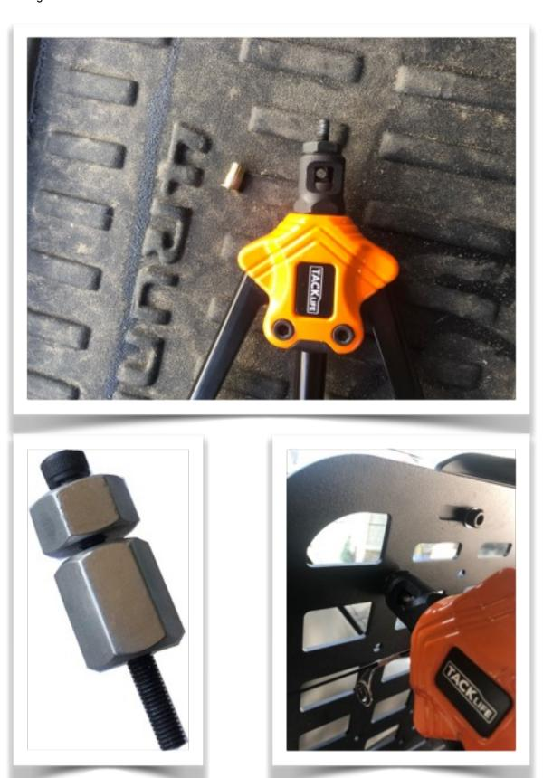
Rivnut is now installed! Refer to 5 b) to finish installing your Barrier.
