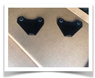
The photo below shows the correct positions. Left is drivers side Right is passengers side. When sliding the brackets on, using a silicon or some type of lube helps slide the brackets on easy without much effort. Put the head rests with the brackets installed back into seats. (Note: when removing the panel you do not need to remove these brackets. Seats will fold down with them in place)
