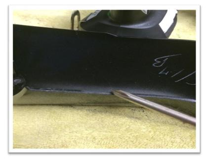
8. Place the outer shroud onto the grill. Start at one side and work your way around the grill screwing it
