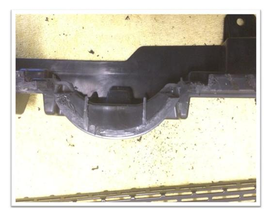
4. Next cut out the remaining plastic and clean up the edges. Doesn't have to be perfect; it will be hidden by the mesh. You could add a piece of plastic to fill the gap but you don't have to, the mesh will hold it firmly in place.
