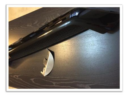
9. Now it's time for the bumper cap. This can be a bit scary. Start but sanding down the paint where the filler will be applied.
