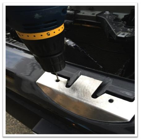
11. Add the spacers before screwing down the bumper cap.
