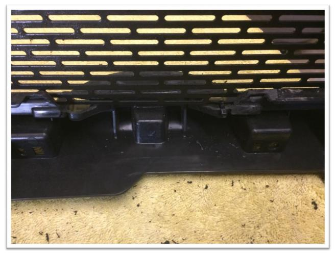
7. The outer shroud has these small tabs that stick out. You will need to grind/Sand them flat.
