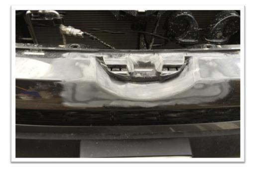
10. Line up where the bumper cap will be mounted and drill some pilot holes.
