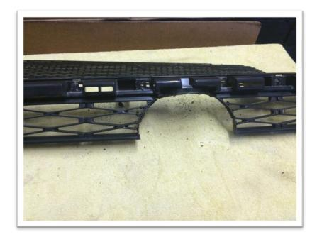
3. Next you will need to notch a small spot for the mesh to slide into where the mesh will be going.
