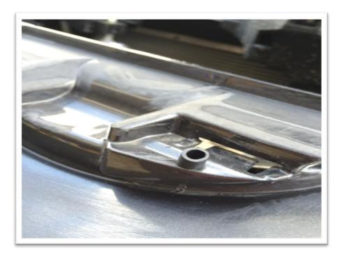
12. Screw down the bumper cap. Make sure all points of the cap are lower than the bumper. You can fill the small gaps with JB weld before using body filler. Once dry, you can begin to add filler.
