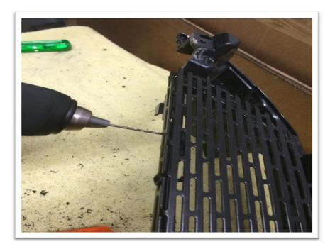
6. After screwing in the mesh. I like to add a small zap strap to help hold the mesh in place, before attaching the outer shroud. Seen here on the bottom right, after drilling a small hole for it to go through.
