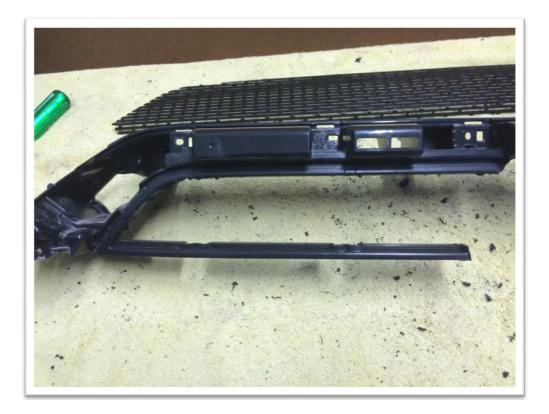
5. Line up the mesh so it is centered on the grill. Then drill a small pilot hole for the mounting screws. Two on each side will be fine.
