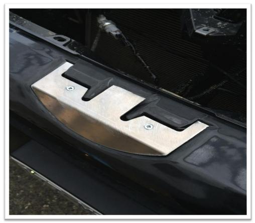
13. You can unclip the lower bumper mesh to protect it from the filler and later from paint.
