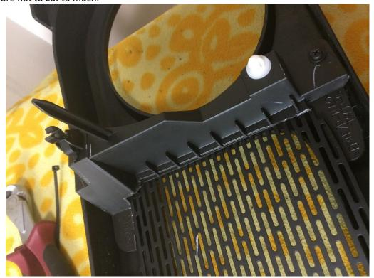
8) Once trimmed you can use nippers to trim the tabs on the inner grill, so that it will sit flat against the mesh. Once done you can put the two trimmed grill pieces back on using the Philips screws (removed earlier).
