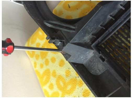
2) Next, using a Flat-headed screwdriver separate the two grill pieces by pushing back all the tabs, working you way around the grill.
