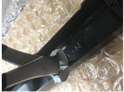
4) Using a Dremel or a rotary tool, sand down the tab enough to make if flush with the rest of the grill. You want to take off just enough so the mesh will sit flat against it.
