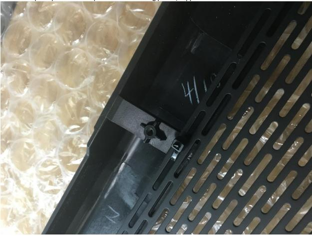
7) You will now need to cut the inner grill like then pictures below. Be sure to test fit frequently to insure not to cut to much.
