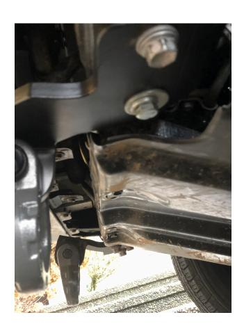
You can see in the photo below how thin the OEM metal is. It is important to remember that the weakest leak won't be the tow hook or the bolts but the frame of the truck. When doing a recovery you should do it from the rear whenever possible. If the front tow hook needs to be used you should split the load with the other side using our Passenger side tow hook mount for the safest recovery.
