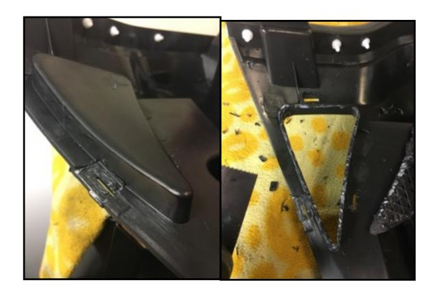
Now clean up your edges. You can use sand paper if you plan on painting. Most of the melted plastic will come off by hand so you could get away with out painting. If you are painting be sure to clean the grill with some rubbing alcohol first. Use masking tape over the rubber seal.
