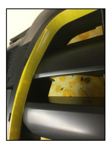
Using 3/4 inch electrical tape, Tape the lip around the grill. This will be your cut line so make sure you have it exactly where you want it.
