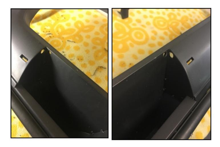
Clean the working area and start zap strapping the mesh into place. Install all the zap straps before pulling them tight. Once you have done that line the grill up and start tightening them all the way around.
