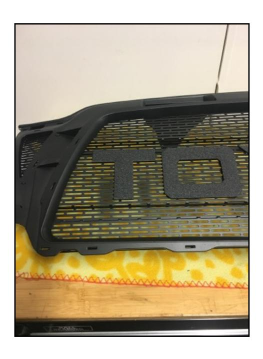
You can now install the outer shroud. We recommend installing the same way you removed it by melting the two grill parts together. This can be done with a soldering gun, just make sure the two parts are tight together. You could also use JB plastic weld.
