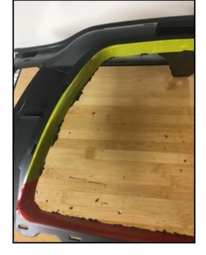
You can now move on to the triangle portion on the grill sides. We are using a multi- max but you could also use the Dremel tool with cut off wheel again. Be very carful not to cut too much, were only taking about an 1/8in.
