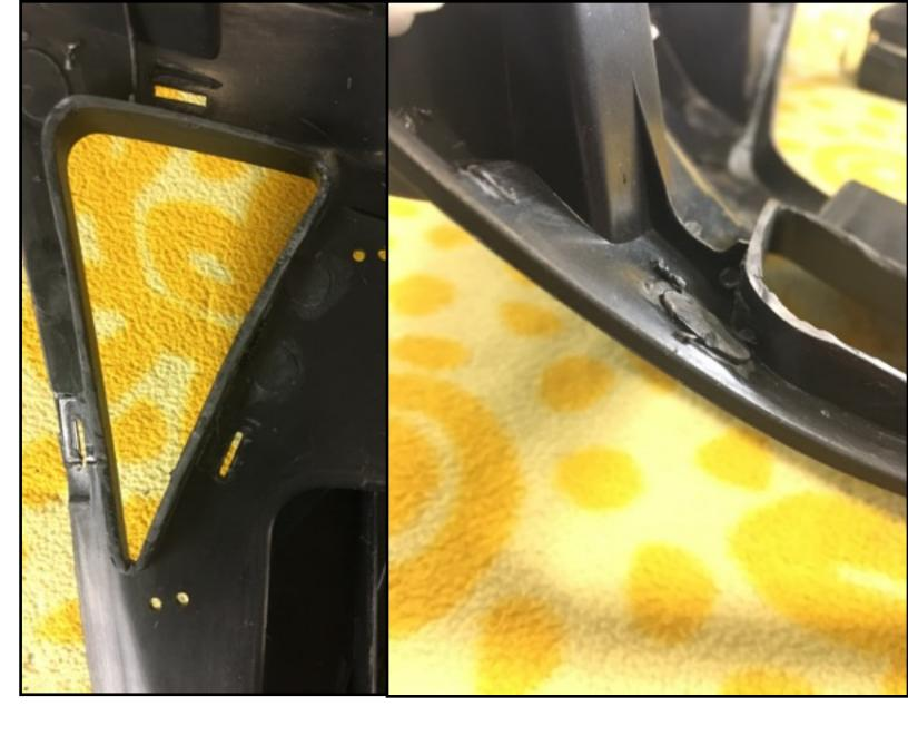
You want to drill these next holes near the front of the grill so that it will put the mesh down. for the large centre mesh just make sure your holes will line up with a spot with a closed slot.
