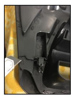
Using razor blade cut off the hight parts of the melted tabs. (You can also use
