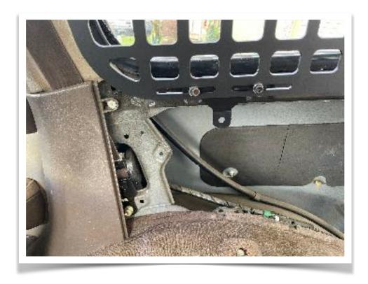
6.) You can install the bottom two brackets leaving them slightly loose. Push the panel against the truck. Using a marker, mark the two hole locations.
