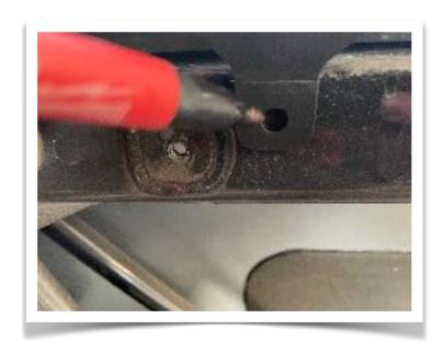
7.) You can now drill the marked hole locations. You may find it easier to remove the panel to drill these holes.
