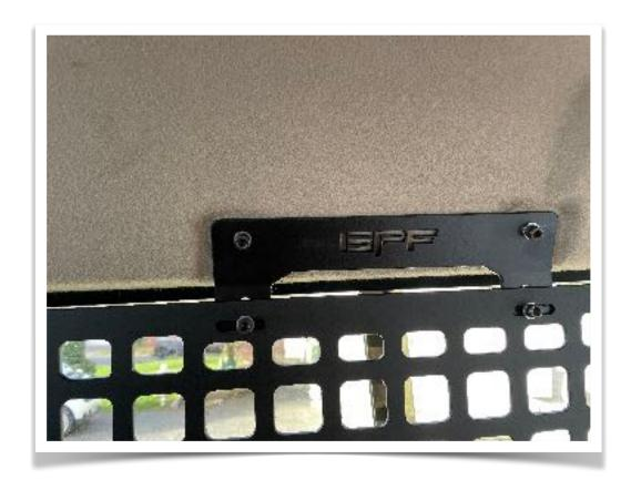
5.) You can either mount this over the OEM plastic or you can pull the cover off and mount it behind. (*Note: the cover will stick out more doing it this way. You also may need some foam to prevent any rattling.*) We will show you with the cover removed as the install method is the same if you mount it over the covering. Start by pulling a corner of the cover off and work your way around, until you have it removed.
