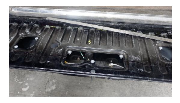
3. You can now lay the new panel on to the tailgate. Put **all** button head bolts into their hole locations. This will aline the panel so you can draw out where you will be cutting.
