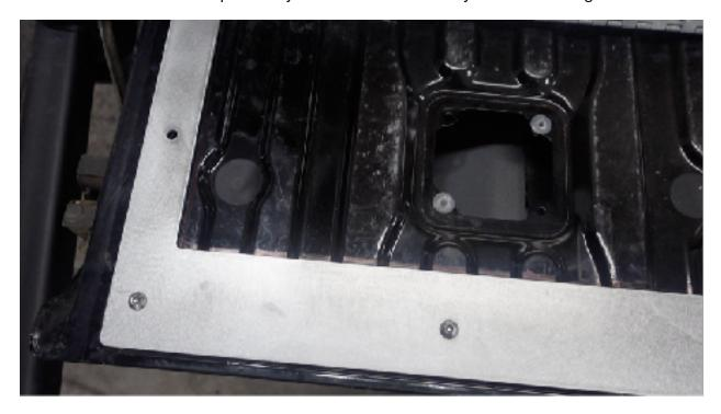
4. You want to leave a 1/4 inch of the original tailgate on the sides and the top portion (area closest to you when the tailgate is opened). On the hinge side you will be removing extra material to accommodate for the hinge bolts. This is what the new inside panel will be sitting on. It will be better for it to be on the bigger in size so don't go crazy cutting you can always trim more after.
