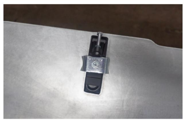
9. With the hardest parts completed, you can now remove the tailgate panel and vacuum out any of the dust and metal left behind. If you have it or want to install sound deadening material, now is a good time to install it.
