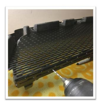
Set the mesh on top of the grill and line up the edges. You can then drill a 1/8 pilot hole to attach the first screw.
