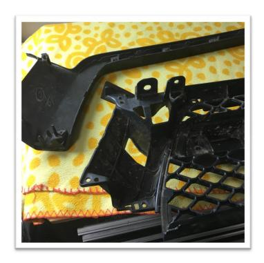
Carefully pull the shroud off the grill frame making sure all screws are out and all clips are released.
