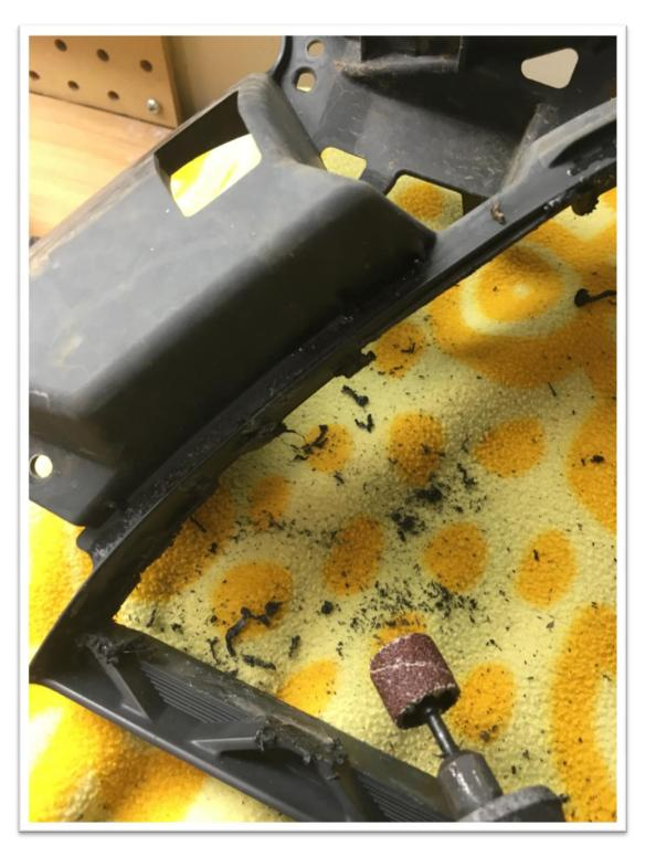
You can use the Rotary tool to clean up any messy cuts and smooth down the edges.
