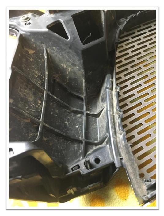
Confirm the mesh still lines up and hasn't shifted. You can now join the outer shroud with the frame. Attach the screws back into the grill before clipping back into place. Once screws are in place you can now tighten them up and clip the grill back together.
