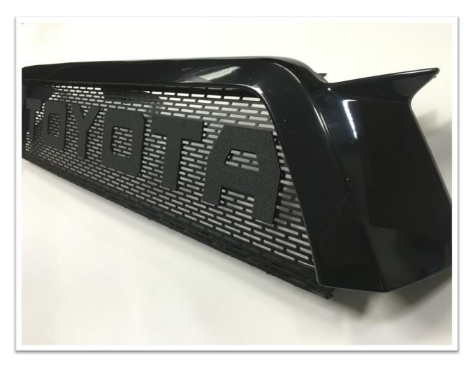
When installing back onto the truck we like to add masking tape to the upper bumper where the screws are to help prevent scratching.
