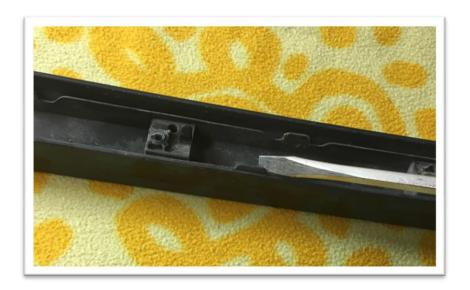
Set the painted shroud on a soft clean towel or blanket. Using a Rotary tool, grind down the tabs on the back of the shroud.
