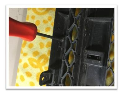
Using a Philips screw driver remove all screws from the grill.
