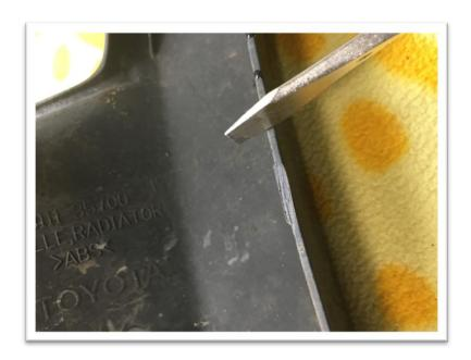
Grind down the tabs just enough so that it is flush with the rest of the grill.
