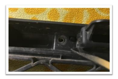
Using a Flathead screwdriver, push back the plastic tabs. You can then unclip the painted shroud from the grill frame.
