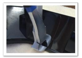
5. Smooth the sharp surfaces from the clipped tabs with a Dremel or sanding tool. Set grill frame aside.
