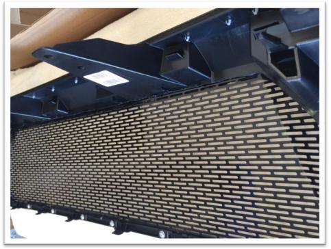
12. Bend the high points of the mesh on either side down, so that you will be able to clip the piece together with ease.
