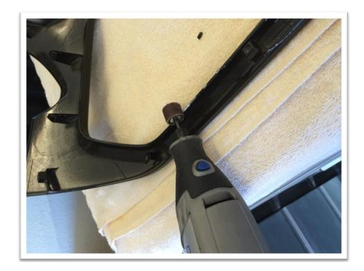
6. On the other piece from your original grill (inner shroud), use a Dremel or hand saw to cut the middle from the outer portion.
