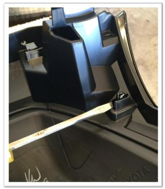
4. Locate the tabs on the inside surface of the grill frame, and remove them using nippers
