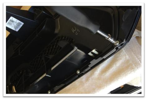
3. Using a flathead screwdriver to open the clips and separate the outer frame of the grill from the inner shroud.
