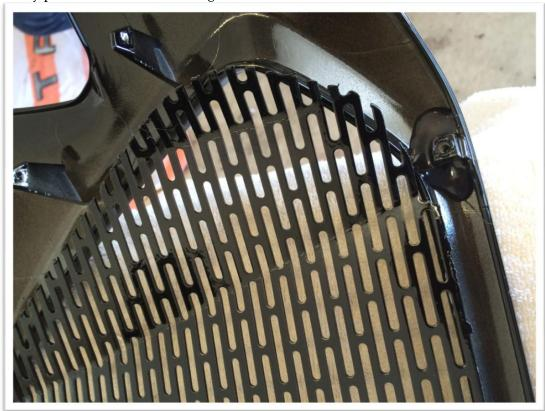
11. Place the inner shroud overtop the mesh that is mounted on the outer grill frame, lining it up to the clips and screw placements. Now make sure the mesh is level.
