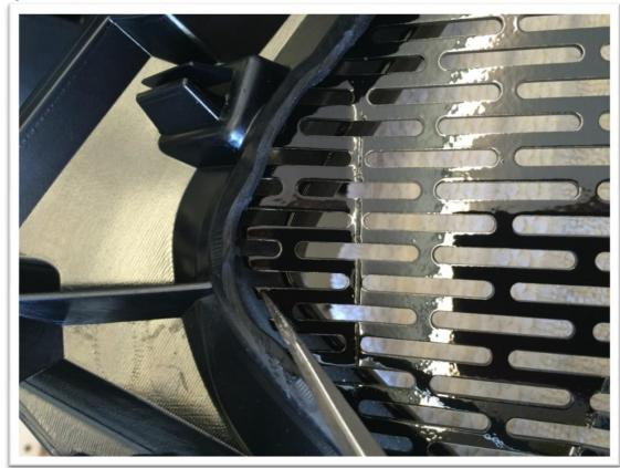
13. Screw together the inner shroud to the outer grill frame with the mesh in between. Next, clip the piece together. For best assistance, use pliers for added force.
