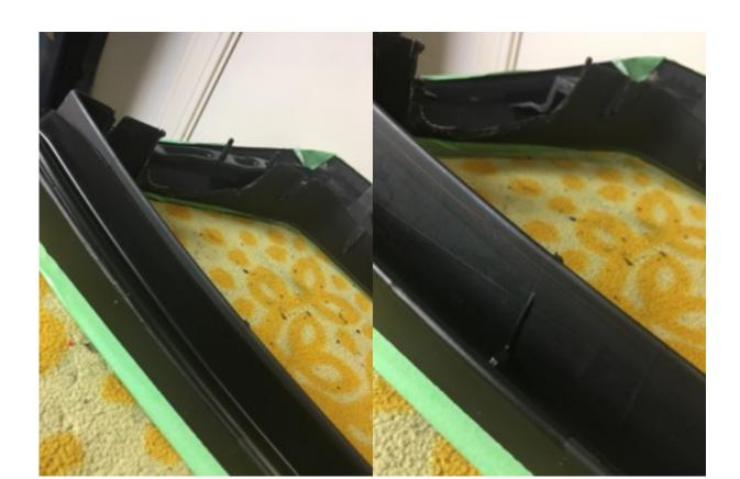
4. Once you have the mesh sitting flat you can cut out some notches for the mesh to slide into.
