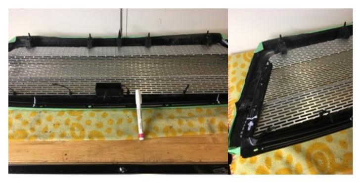
8. Next you can drill some holes in the lower hood latch bar so you can attach the mesh later. Once done be sure to paint any bare metal. You can also see in the photo blow how you will need to notch the mesh so it will allow for the bar to sit flat.
