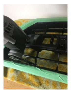
3. You will need to cut the grill lip making it as flat as possible. You can trace a line using the metal hood latch bar. You can test fit the mesh and see how flat it will late. If its not sitting how you like you can trim or sand down the higher edges. We use a rotary wheel on a Dermal, but you can use a sander. Our lip on the sides worked out to be an 1/1/4.
