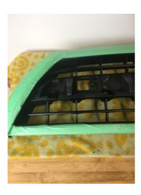
2. Next Cut out the centre of the grill using a Multi-Mar or a hand saw.
