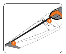
Moving from bow to stern, unclip the fairings and remove the foam plug. Unbuckle and loosen every side-release buckle and clip. Unbuckle the tension strap. Do not loosen the end straps yet.
