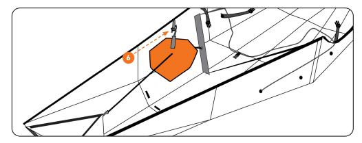
The bow bulkhead stays in the kayak. Hook it onto the gray ring strap as shown. This keeps the bulkhead and footrest safely out of the way when folding up the kayak
