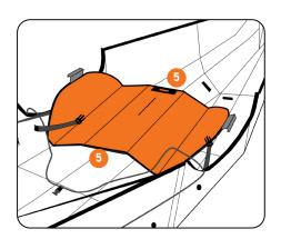
From the center sides on the rubber trim indicated in the illustration above. Do **not** use the bungee to remove the floorboard.
