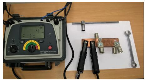
a skewed connection, caused by improper tightening of the bolt, is included. These examples illustrate that while basic continuity testing has a vital place in the electrical maintenance spectrum, there are many instances where a developing problem would show up only as a falsely reassuring "0" on a multimeter whereas a rigorous low resistance test would boldly expose it.
