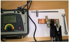
where electrical current is involved. Overtightening can cause the connection to become skewed, with less surface contact and higher resistance.
