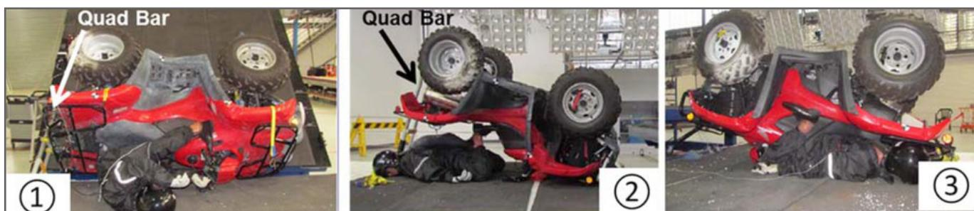
Rollover Tests: (1) crush protection provided when the Quadbar serves as an anti-roll bar in a side overturn, (2) the clearance provided by a Quadbar for the dummy in a forward overturn, and (3) a dummy crushed in a forward overturn without a CPD. Source: Grzebieta et al. 2015. (7)
