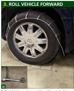
Roll vehicle forward over cable until beaded cable ends are are positioned midway on the tire and keyhole latch (3A) is easily accessible.
