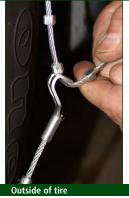
4B. Place beaded cable end through keyhole latch and pull to tighten.
