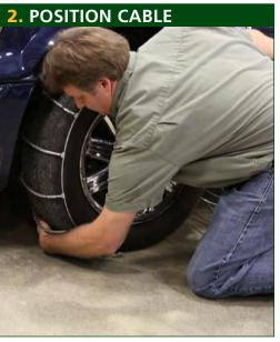
Position cable to be centered on tire treads. Straighten cross cables to lay horizontal across tire treads. Tuck first cross cable under the front of your tire in preparation to roll over them.
