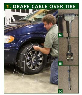
Drape cable over tire after laying cable flat by tire and inspecting it for any kinks. Set cable etched TIRE SIDE (1A) against the tire wall. Place the keyhole latch (1B) toward the front of the tire, and beaded cable ends (1C) toward the back of the tire.
